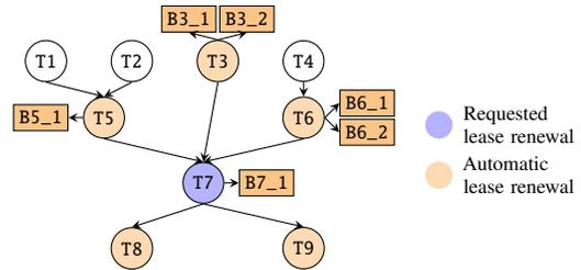
**Fig. 5. Lease Renewal via Address Hierarchy.** Hierarchical addressing simplifies lease renewal in Jiffy (§3.2), since lease renewal for an address-prefix automatically implies renewals for all parent and descendent address-prefixes in the hierarchy.
