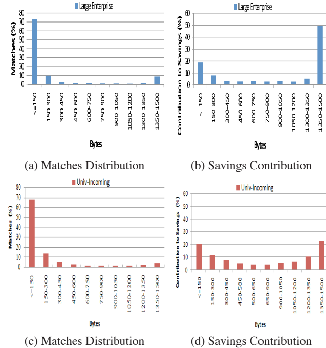
Figure 8: Match Len Distribution and contribution to total savings. (a) and (b) are for large Enterprise. (c) and (d) are for University Inbound traces.
