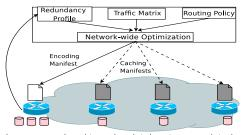
Ingress encodes pkts and maintains stores per interior-router Interior routers cache a subset of pkts acc. to their manifests Ingresses generate and report match profiles to the NOC
