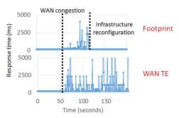
Figure 8: Testbed experiment: WAN congestion.
