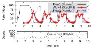
Figure 16: Support for bandwidth stability
