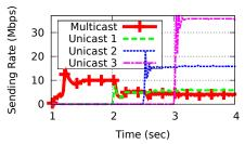
Figure 18: Multicast flow adapts to congestion.
