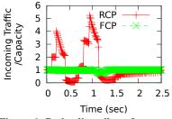
Figure 6: Preloading allows fast, graceful convergence.
